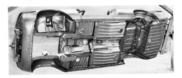
of the 2000 model—and many other design changes were required, so that virtually new sub-assemblies were evolved as a basis for the body. The only pressings in the final design that are common to both models are the front longitudinal members, one transverse member in the floor, the front valance assemblies, and stiffeners for the rear wheel-arches.
