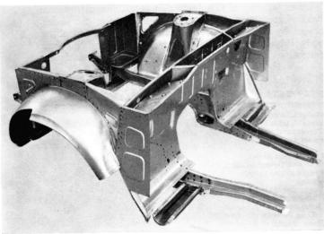
Top: Fabricated 0.064 in thick pressings comprise the front longitudinal box-section members that carry the engine, the lower pivots for the front suspension, and the steering gear. The front valances are reinforced for the upper mountings for the suspension
