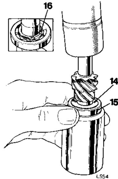
17. Fit water pump body in small hole of 348/1.
