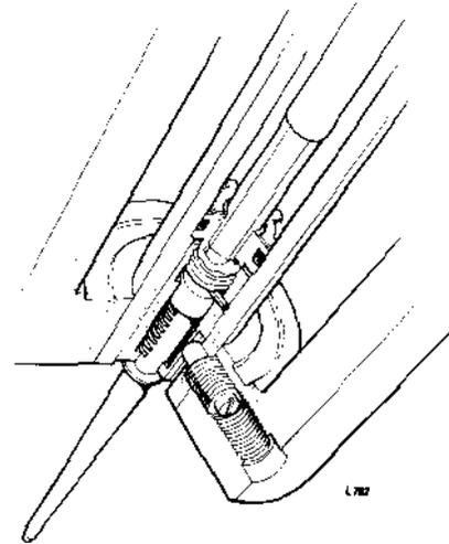
35. Fit diaphragm, locating inner tag into recess in air valve.
