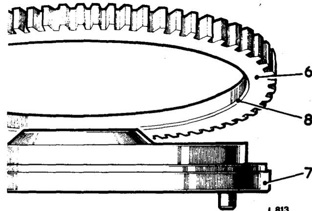
9. Allow the ring to cool gradually to avoid stress distortion. A maximum permissible gap of 0.025 in (0.6 mm) is allowed between flywheel and starter ring on one length of 6 in (15 cm) only.
