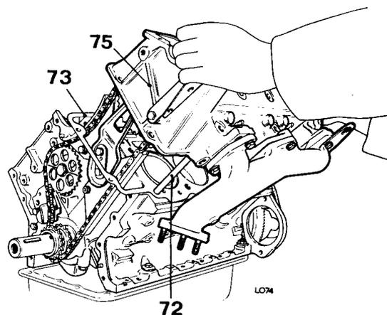
76. Fit remaining cylinder head studs, washers and nuts.
