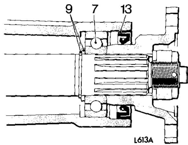
13. Fit oil seal—spring innermost—to extension so that seal wall is flush with extension wall.
