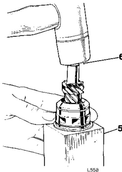
5. Insert assembly, gear uppermost into small hole of 348/1.
