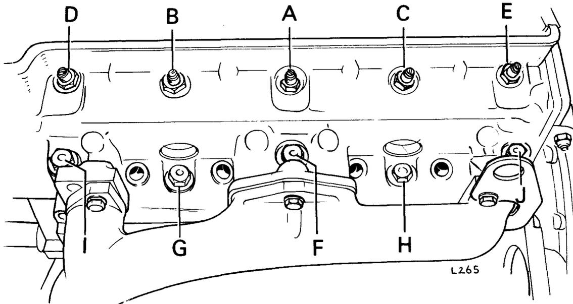
47. Reposition coil; fit and tighten bolts.
