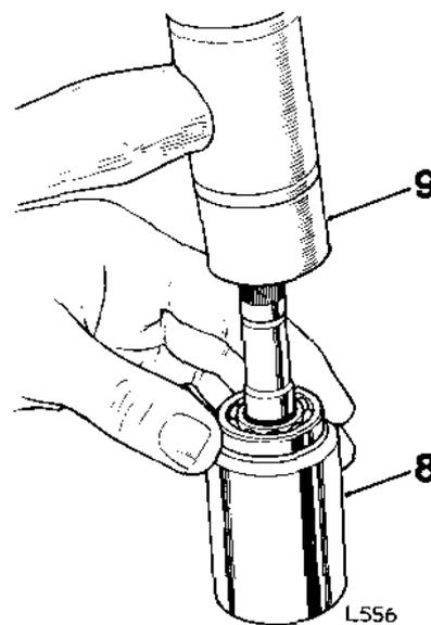
8. Insert shaft, gear down, into 348/7.
