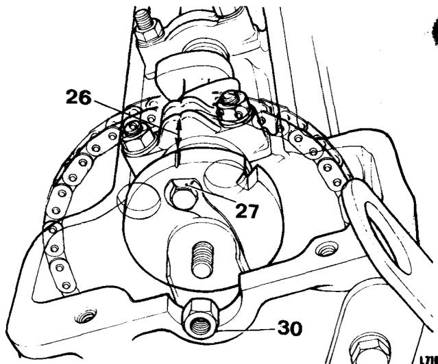
32. Remove three bolts securing water pump cover to cylinder block; remove cover.
