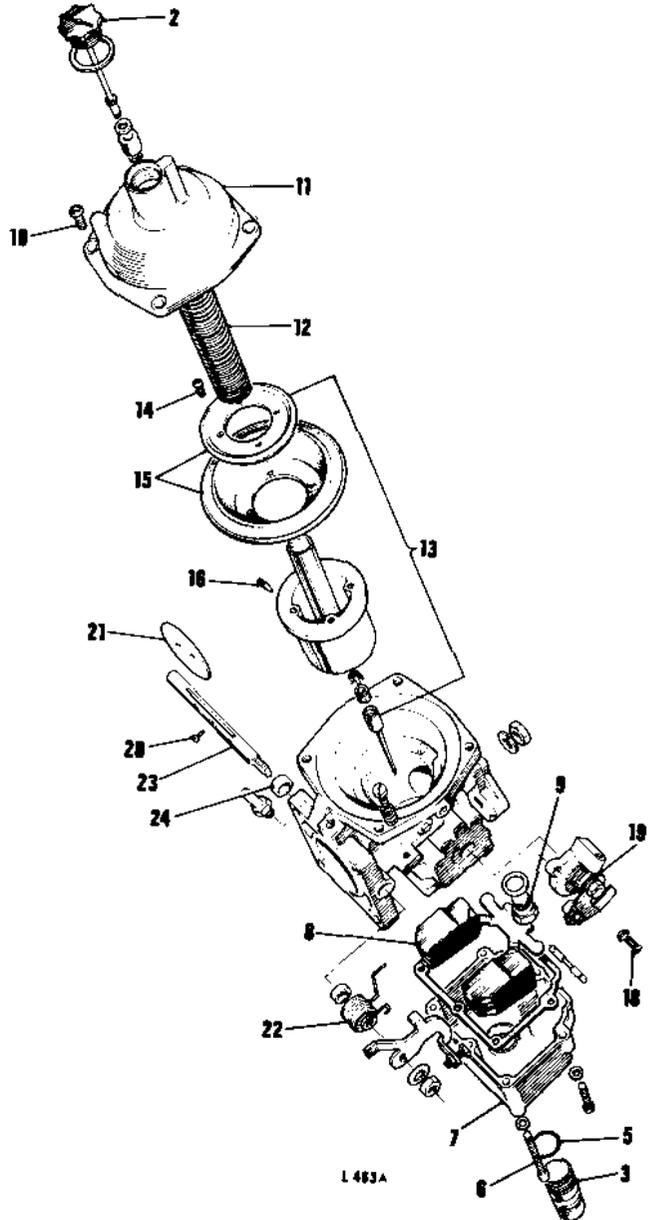
28. Fit spindle seals to body, tapping gently into position, with metal casing of seals flush with body of carburetter.
