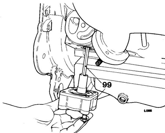
**CAUTION:** To prevent damaging the sump or head gaskets care must be taken fitting the front cover. It is good practice to use strips of shim steel to slot the cover between the gaskets.
