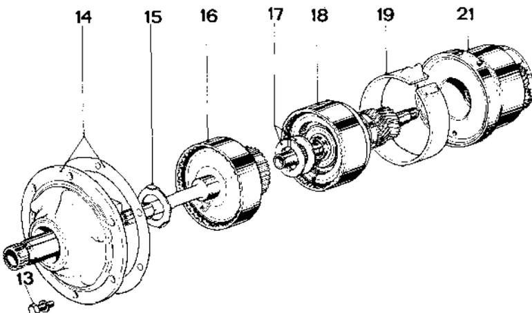
22. Separate the centre support from the planet gear assembly.
