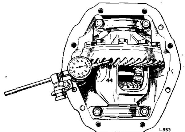
44. Using dial gauge, check backlash at several points on crown wheel. If a mean reading outwith 0.004 to 0.006 in (0.1016 to 0.1524 mm) is obtained, transfer shims from one carrier bearing to the other as required.
