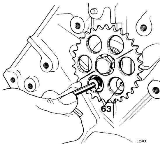
63. Fit jackshaft keeper plate and secure with two countersunk hexagon recessed screws.
