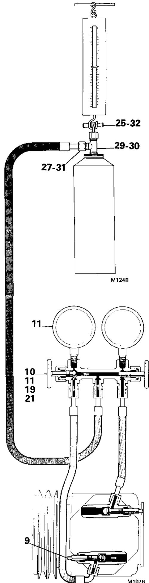
35. Slightly loosen hose connector at centre manifold connection to allow refrigerant to purge air from centre manifold hose. Tighten hose connector.
