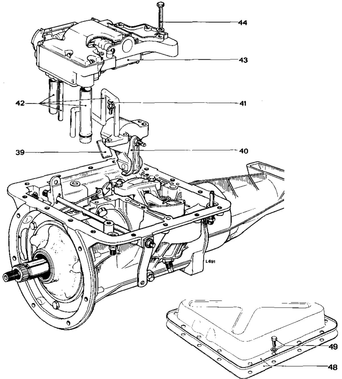
39. Using petroleum jelly, stick the front strut to the front servo lever.
