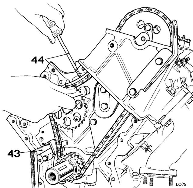
45. Fit R.H. bank camshaft gear with one bolt and lockplate.
