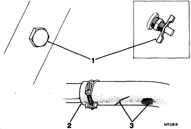
**(35) Evaporative and crankcase ventilation systems—check hoses and restrictors for blockage, security and deterioration.**
