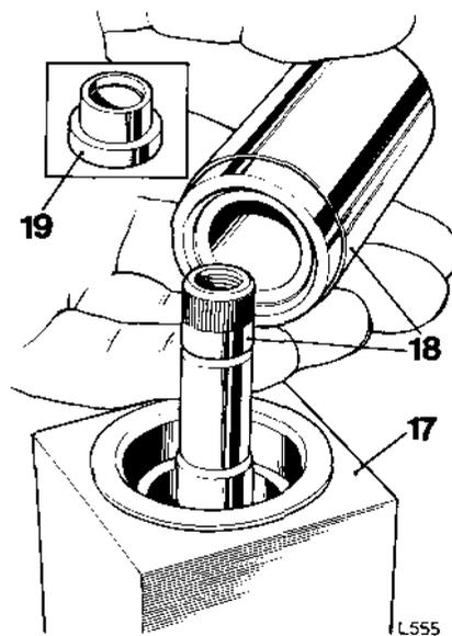
20. Fit water flinger dish towards bearing, using tool 348/2.
