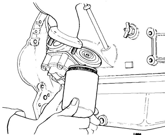
**OIL FILTER ASSEMBLY—EXTERNAL****—Element—remove and refit****12.60.02****—Overhaul****12.60.08****Working below the vehicle:**
