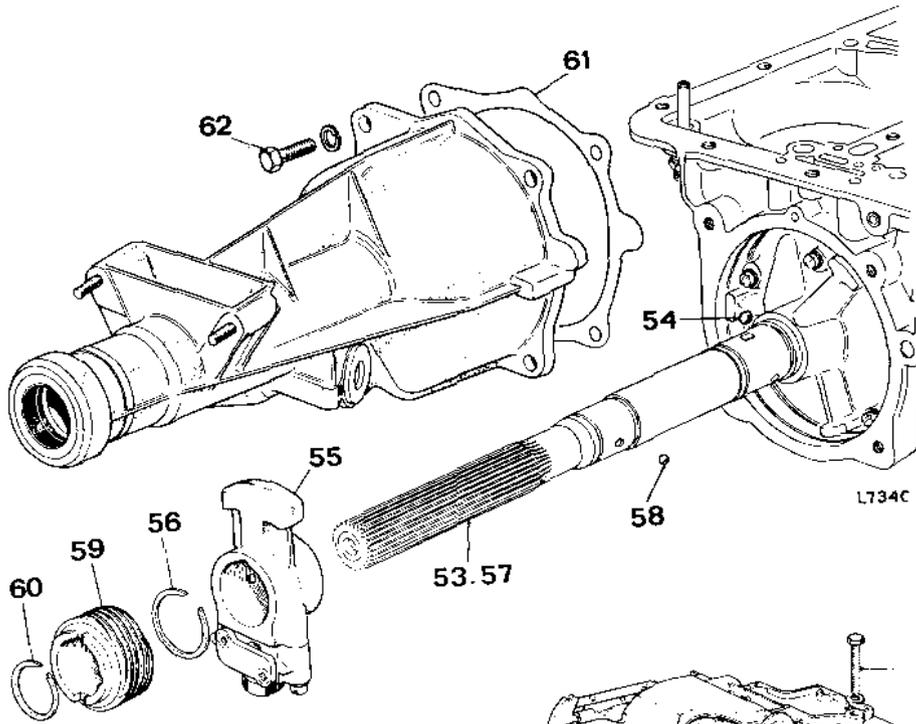
53. Turn the output shaft until the governor drive ball detent is uppermost.
