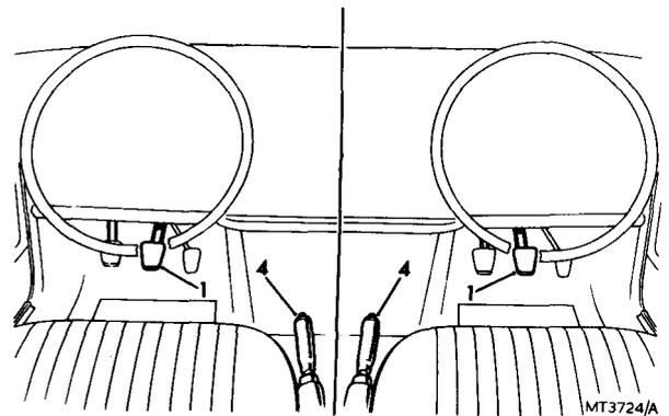
**(68) Check/report brake pedal travel and hand brake operation.**
