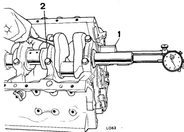
1. Fit magnetic dial gauge indicator to front of cylinder block with indicator rod on end of crankshaft.
