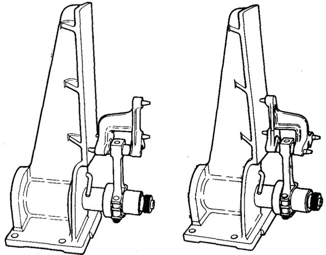
**CAUTION:** The connecting rods are offset and chamfered on one side only; this side fits adjacent to the crankshaft. Thus each pair of big-ends are fitted to the crank journal with **non-chamfered** sides together.
