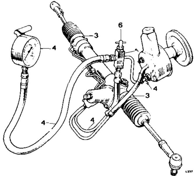
11. With engine idling, turn steering-wheel gently to left and right, observing gauge reading. **DO NOT** hold wheel in either direction for periods exceeding five seconds. Check that pressures of 52.73 to 59.76 km/cm<sup>2</sup> (750 to 850 lb/in<sup>2</sup>) are obtained in both directions.
