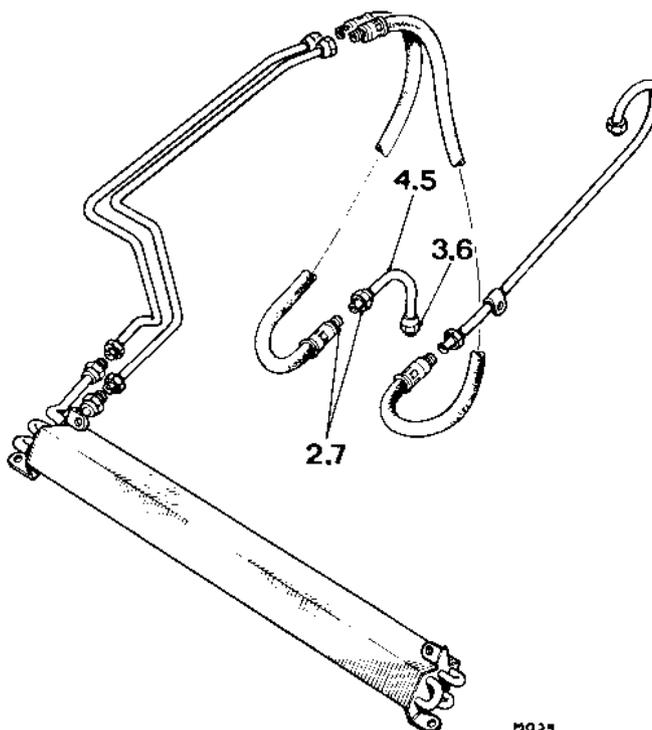
**OIL COOLER PIPES—Gearbox End Return Pipe**
