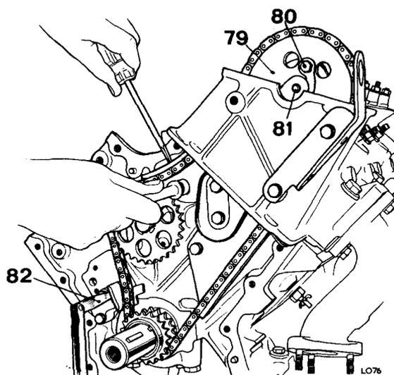
84. Fit outer chain tensioner, keeper and spacer. 12.65.29.
