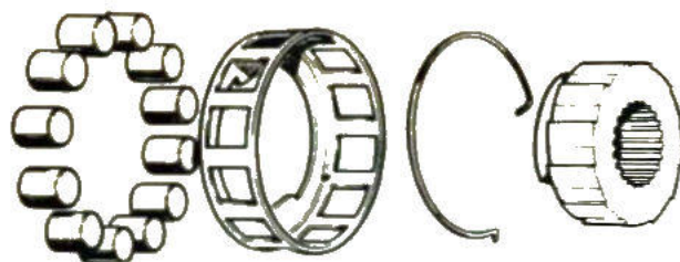
FIG. 25. UNI-DIRECTIONAL CLUTCH COMPONENTS
